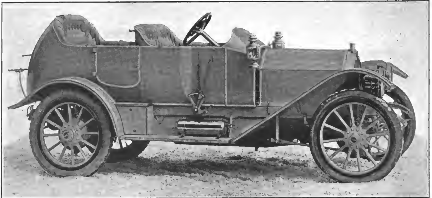
Right side of torpede model, showing side levers conveniently arranged outside of body line, with depression in body to accommodate them
